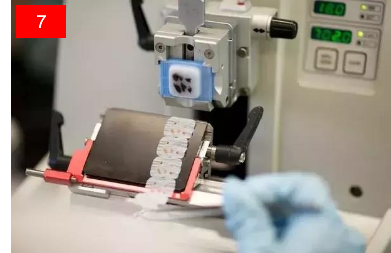
Thin sections are cut on a microtome
